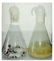
Fig. 3 Hydrolysis of paper cup
